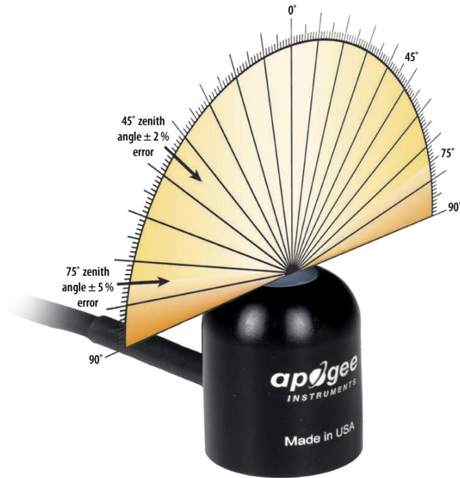
Directional, or cosine, response is defined as the measurement error at a specific angle of radiation incidence. Error for Apogee SQ series quantum sensors is approximately  $\pm 2\%$  and  $\pm 5\%$  at solar zenith angles of  $45^\circ$  and  $75^\circ$ , respectively.
