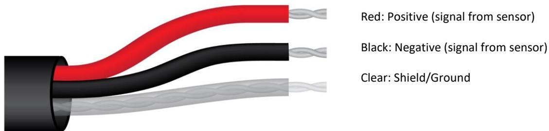
Wiring for: SQ-110 and SQ-120 Serial Numbers 25370 and above
